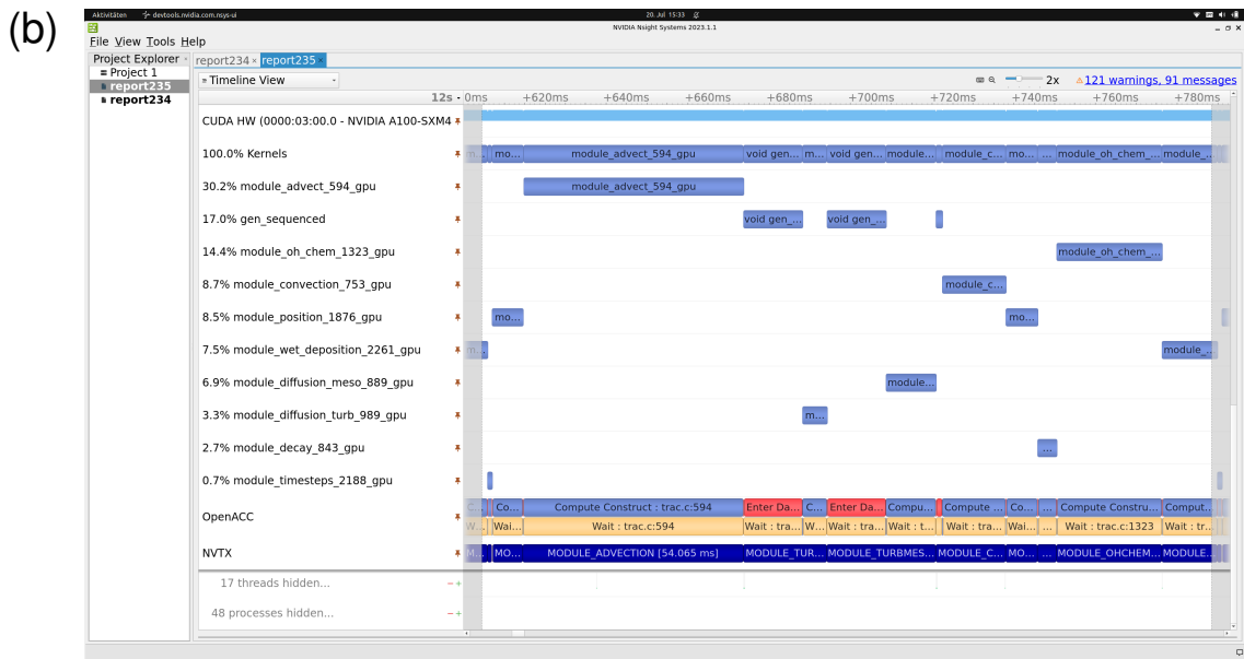
Figure 2. Timeline analyses of a single time step of the MPTRAC Lagrangian transport model for a simulation with 10^8 globally distributed air parcels driven by ERA5 data. Results are shown for (a) the baseline code of MPTRAC and (b) an optimized code version with improved data structures and memory access patterns. The analyses were conducted on the JUWELS Booster HPC system at the Jülich Supercomputing Centre, Germany. The Nsight System report files used to create this figure are made available in the electronic supplement to the paper.
