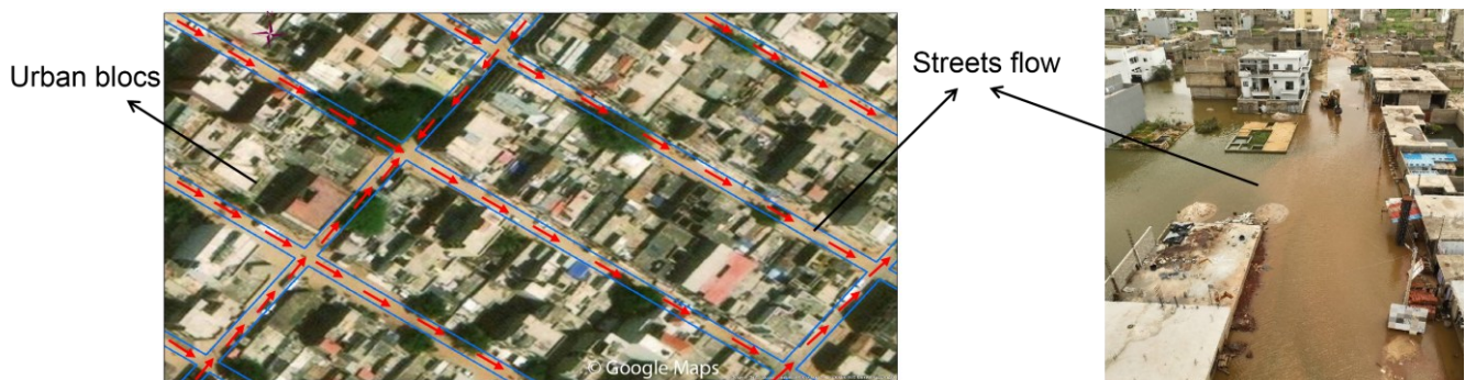
Figure 7: Surface water drainage paths at urban street level.
