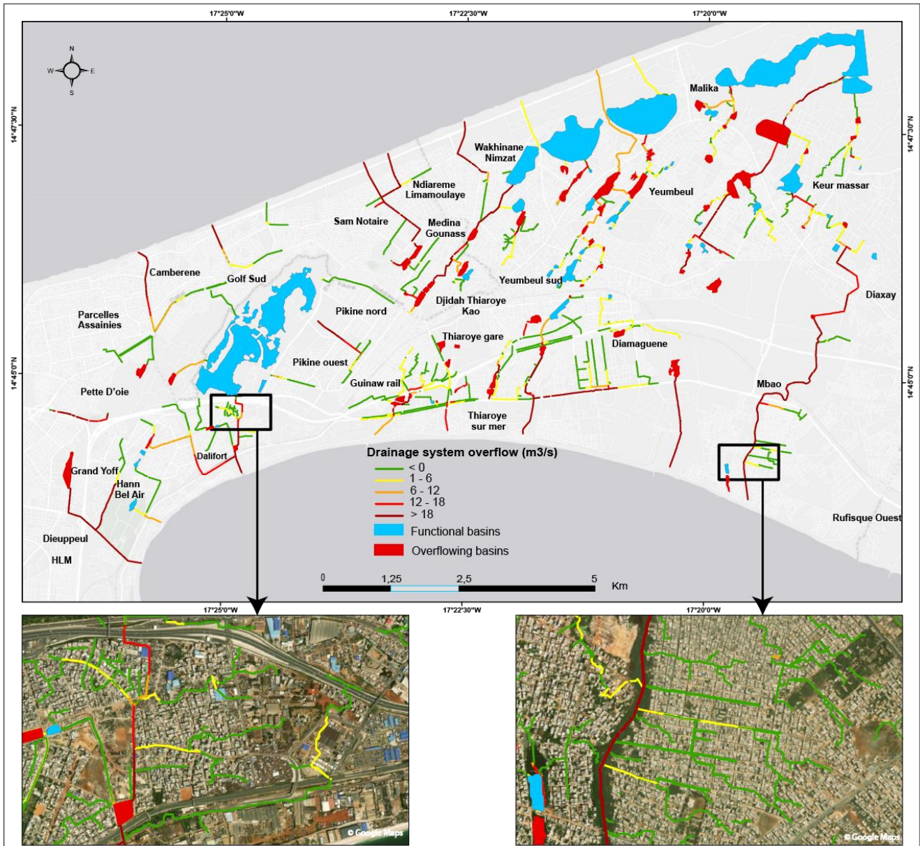
Figure 11: Identification of network overflow points for a 100-year return period rainfall.
