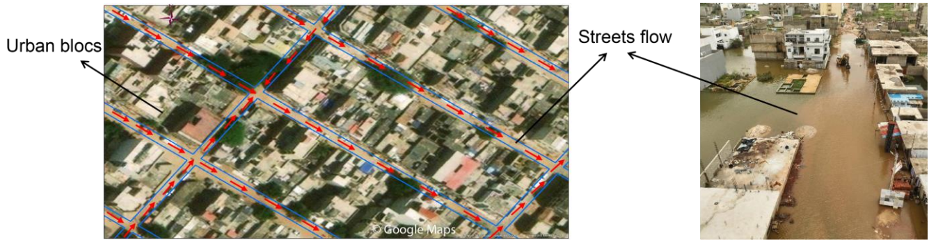
370 Figure 67: Surface water drainage paths at urban street level.
