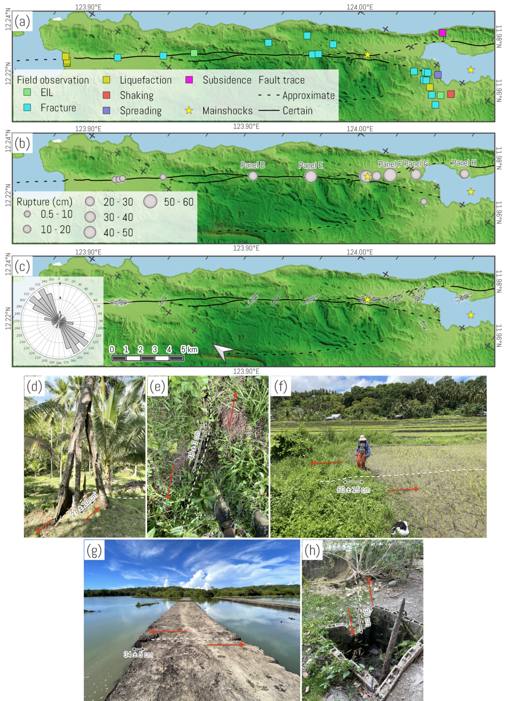
Figure 10. Compiled ground-truthing data. A) Earthquake hazards aside from ruptures. B) Ruptures symbolized by size showing the amount of slip. C) Rupture orientations. D) Ruptured tree showing cumulative 87 cm slip from 2003 and 2020 events with estimated 27 \pm 10 cm offset from the 2020 earthquake. E) Soil mound cut by the fault highlighting a 48 \pm 3 cm left lateral offset. F) Rice field embankment traversed by fault showing 60 \pm 15 cm displacement. G) Ruptured fishpond dike recording a 34 \pm 5 cm offset. H) Abandoned septic tank showing a 30 cm displacement south of Cataingan Bay.
