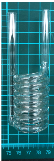
Figure 2: Compact borosilicate glass coil trap, consisting of a 9 mm o.d. x 7 mm i.d. inlet downtube (on the left), connected to a tightly coiled 6 mm o.d. x 4 mm i.d. section with subsequent outlet tube. Scale on bottom is in cm.
