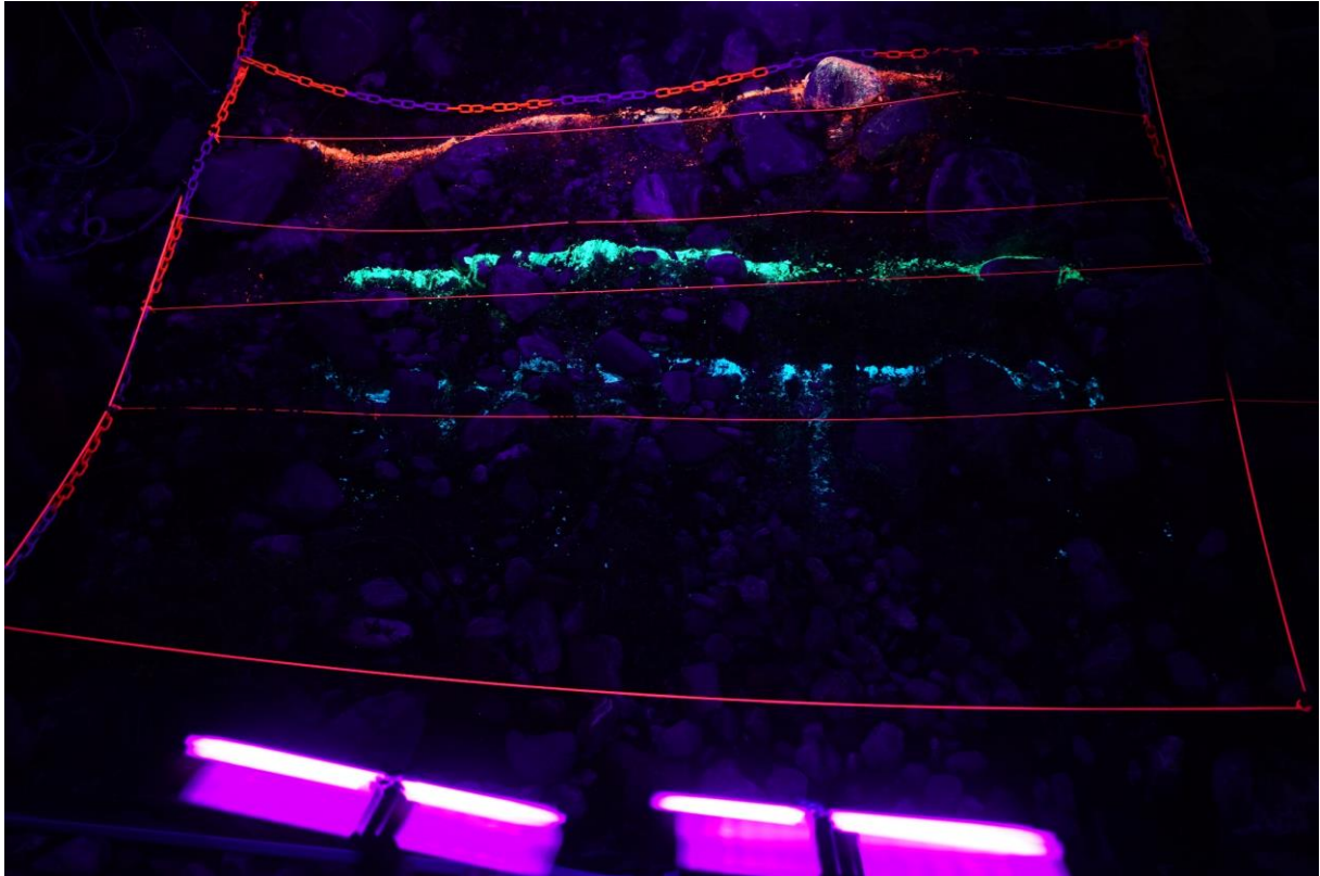
Figure S8: Nighttime photo of the 1990L plot, taken after the high intensity (HI) experiment. The sand was illuminated with two LED lamps before and with six UV lamps (of which two can be seen at the bottom of the photo) before and while taking the photo. The orange sand ribbon was added prior to the low intensity experiments (LI), the green sand prior to the medium intensity (MI) experiments, and the blue sand prior to the HI experiments.
