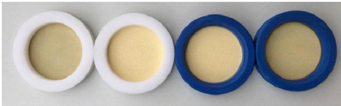
Figure S27: Filters with PM collected from food discards burning; from left to right: Teflon-membrane for PM 2.5 , two Quartz filters in the middle for PM 2.5 , and Teflon-membrane for PM 10 .
