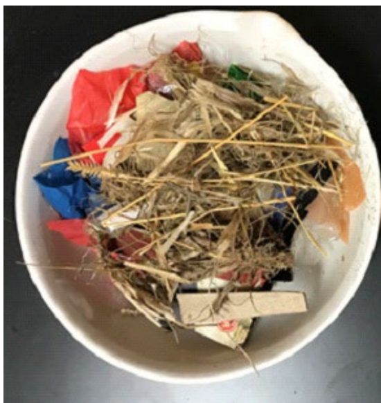
Figure S28: Combined materials in a heated ceramic crucible: a) before burning and b) after burning.
