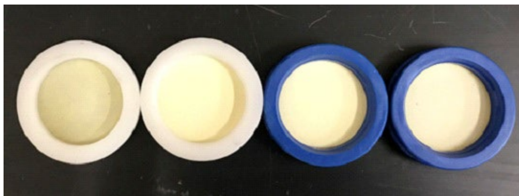
Figure S6: Filters with PM collected from paper burning tests; from left to right: Teflon-membrane for \text{PM}_{2.5} , two Quartz filters in the middle for \text{PM}_{2.5} , and Teflon-membrane for \text{PM}_{10} .
