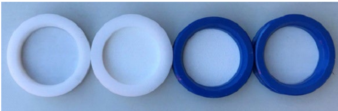
Figure S15: Filters with PM collected from hard plastic (bottle) burning; from left to right: Teflon-membrane for PM 2.5 , two Quartz filters in the middle for PM 2.5 , and Teflon-membrane for PM 10 .
