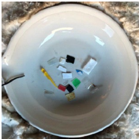
Figure S13: Hard plastic (bottle) material in a heated ceramic crucible: a) before burning and b) after burning.
