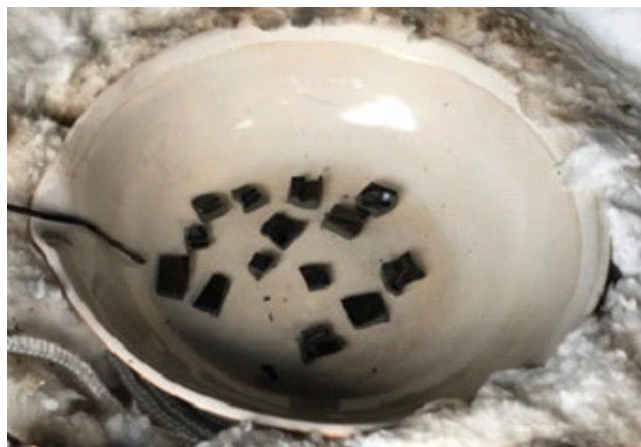
Figure S7: Rubber material in a heated ceramic crucible: a) before burning and b) after burning.
