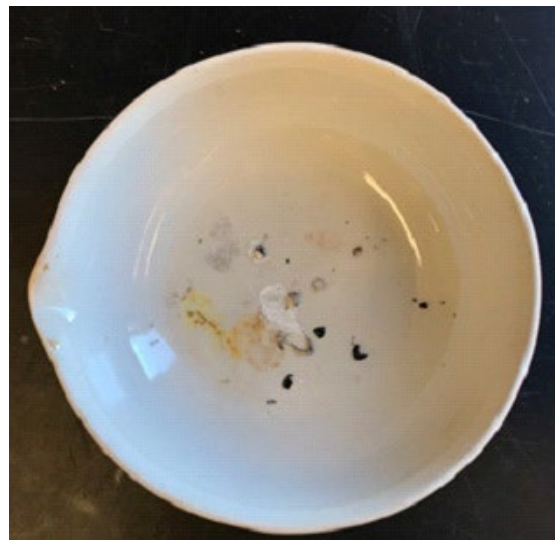
Figure S13: Hard plastic (bottle) material in a heated ceramic crucible: a) before burning and b) after burning.
