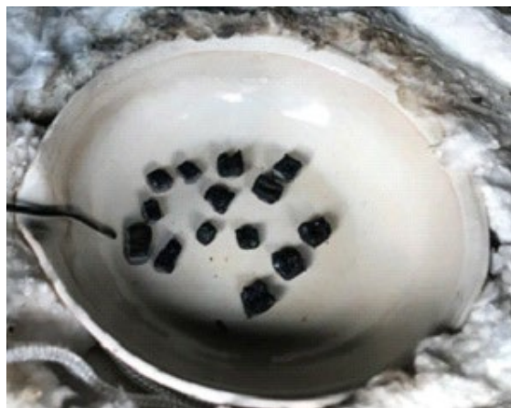
Figure S7: Rubber material in a heated ceramic crucible: a) before burning and b) after burning.
