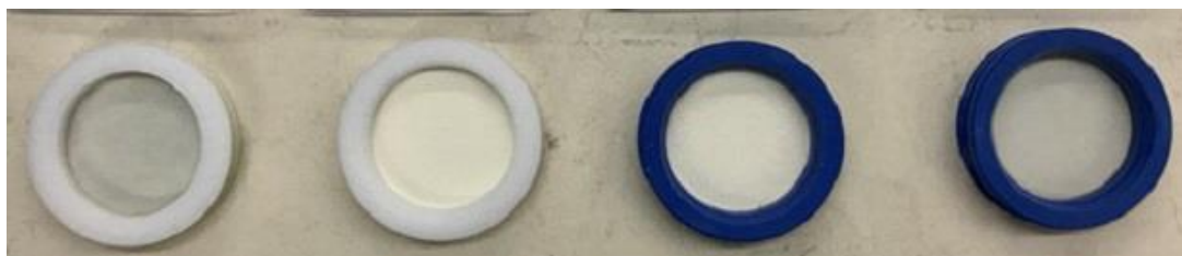
Figure S9: Filters with PM collected from rubber burning tests; from left to right: Teflon-membrane for PM 2.5 , two Quartz filters in the middle for PM 2.5 , and Teflon-membrane for PM 10 .
