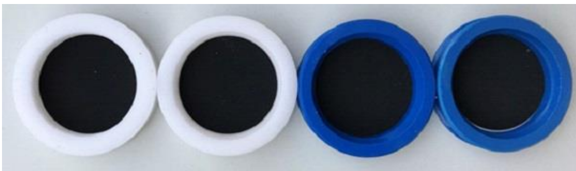
220 Figure S30: Filters with PM collected from a combined materials burning test; from left to right: Teflon-membrane for PM_{2.5} , two Quartz filters in the middle for PM_{2.5} , and Teflon-membrane for PM_{10} .
