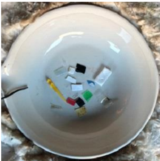
110 Figure S13: Hard plastic (bottle) material in a heated ceramic crucible: a) before burning and b) after burning.
