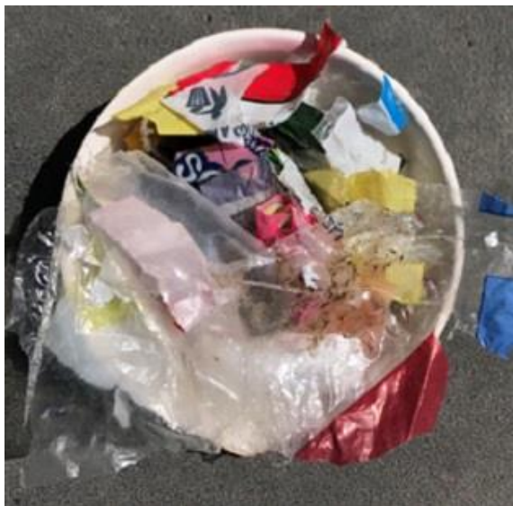
Figure S16: Soft plastic (bags) material in a heated ceramic crucible: a) before burning and b) after burning.
