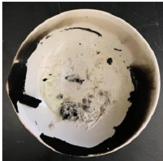
Figure S16: Soft plastic (bags) material in a heated ceramic crucible: a) before burning and b) after burning.
