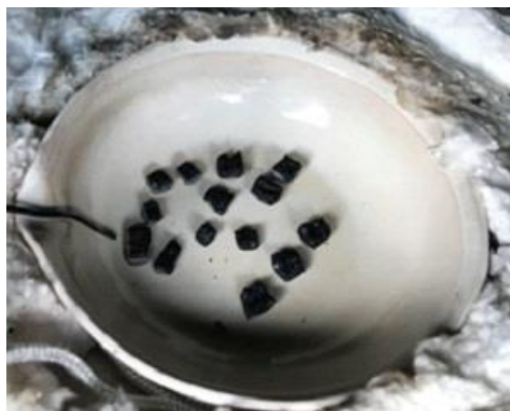
80 Figure S7: Rubber material in a heated ceramic crucible: a) before burning and b) after burning.
