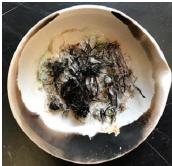
Figure S28: Combined materials in a heated ceramic crucible: a) before burning and b) after burning.
