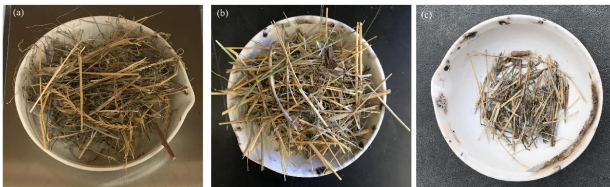
160 Figure S19: Vegetation material, in a heated ceramic crucible for: (a) dry, (b) 20%, and (c) 50% moisture content.
