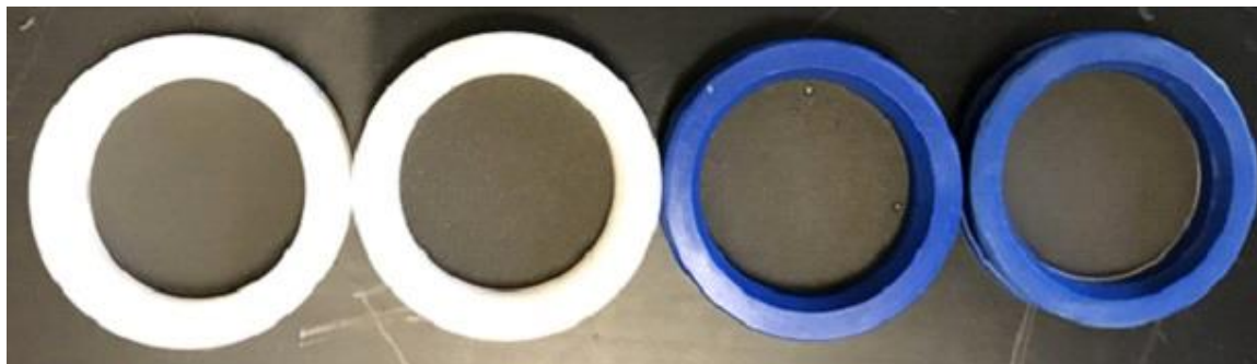
Figure S12: Filters with PM collected from a textile burning; from left to right: Teflon-membrane for PM_{2.5} , two Quartz filters in the middle for PM_{2.5} , and Teflon-membrane for PM_{10} .
