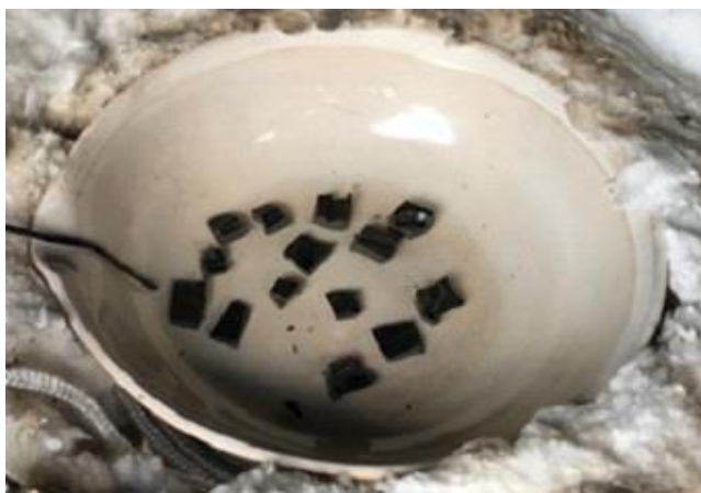
80 Figure S7: Rubber material in a heated ceramic crucible: a) before burning and b) after burning.
