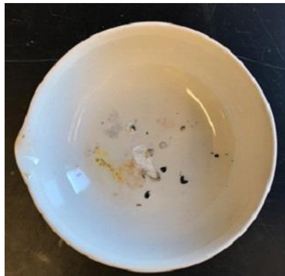
110 Figure S13: Hard plastic (bottle) material in a heated ceramic crucible: a) before burning and b) after burning.
