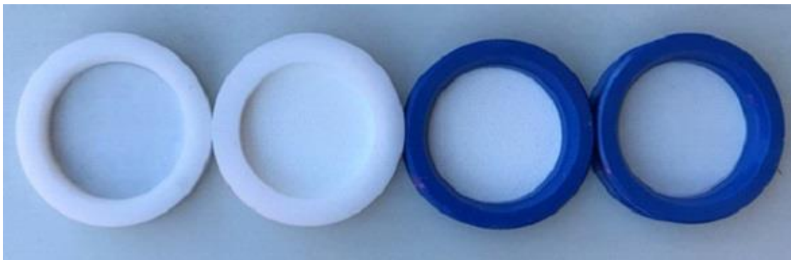
Figure S15: Filters with PM collected from hard plastic (bottle) burning; from left to right: Teflon-membrane for PM_{2.5} , two Quartz filters in the middle for PM_{2.5} , and Teflon-membrane for PM_{10} .
