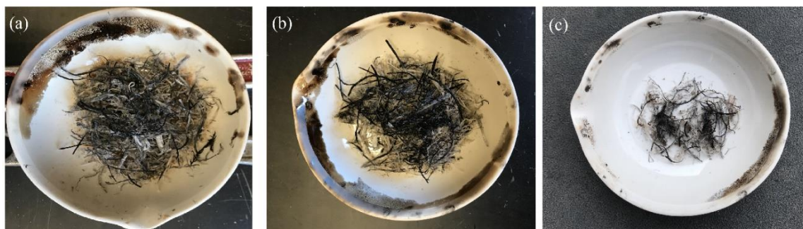
Figure S23: Vegetation ashes for: (a) dry, (b) 20%, and (c) 50% moisture contents.
