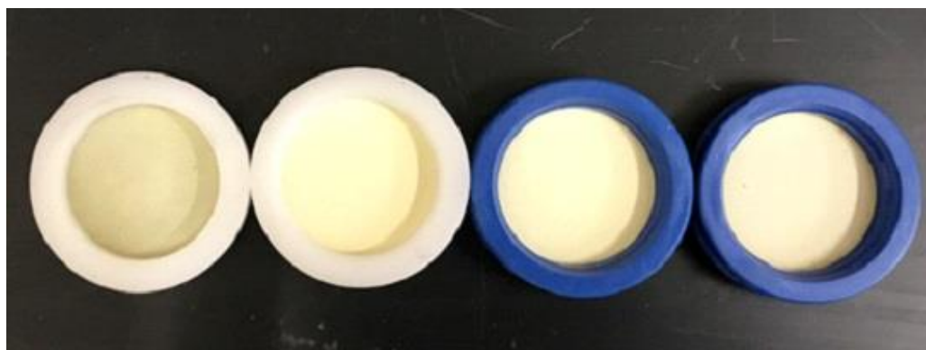
Figure S6: Filters with PM collected from paper burning tests; from left to right: Teflon-membrane for PM 2.5 , two Quartz filters in the middle for PM 2.5 , and Teflon-membrane for PM 10 .
