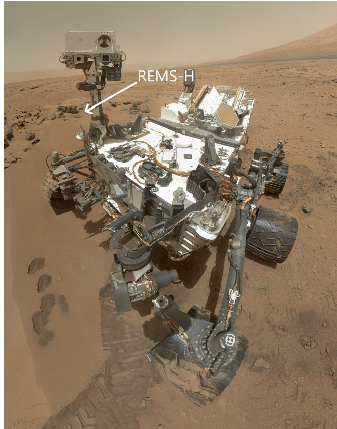
Figure 1. A self-portrait of the Curiosity rover produced by the Mars Hand Lens Imager, which also shows the location of the REMS-H device. (Credit: NASA/JPL-Caltech/Malin Space Science Systems)
