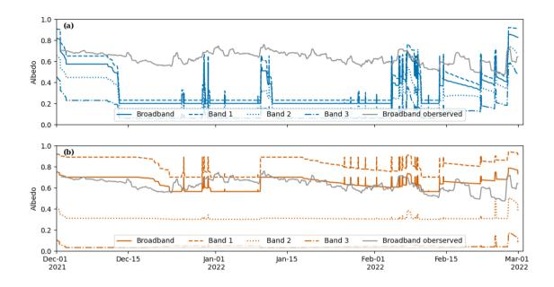
**Figure 6.** Comparison between the daily accumulated broadband albedo in grey and three spectral albedo bands of (a) the original Crocus albedo (oldalbedo) in blue and (b) the modified scheme (newalbedo) in orange.
