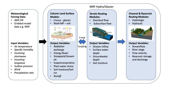
Figure 1. Schematic of the WRF-Hydro/Glacier modelling framework. Modules and variables used in this study are displayed in *italics* and <u>underlined</u>. Adapted from NCAR (https://ral.ucar.edu/sites/default/files/public/WRFHydroPhysicsComponentsandOutputVariables.png, last access: 8 August 2023).
