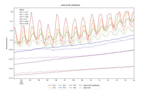
**Figure A2.** Modelled internal ice temperatures from newrunoff\_oldalbedo over the first two weeks of December. Thermocouples were initially deployed at six different depths: 0.05, 0.1, 0.2, 0.5, 1.0 and 2.0 meters. Note that the measurements are not at a constant depth with time as the sensors were melting out over the period.
