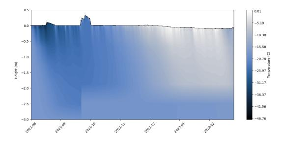
**Figure 10.** Cross section of modelled temperature from newrunoff\_newalbedo of the top three meters of the glacier over the spin-up period of August-November and validation period of December-February. This shows the diurnal variability at shallower depths and the seasonal cooling then warming wave below.
