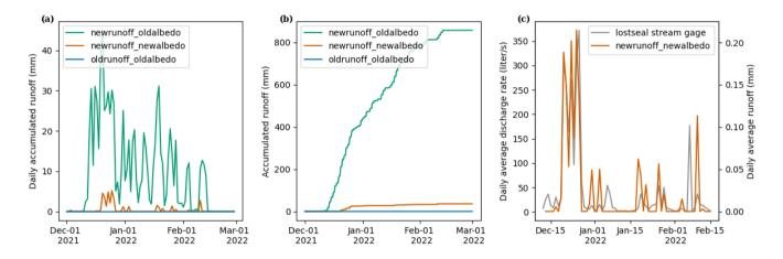
Figure 12. (a) Daily accumulated runoff and (b) cumulative runoff from the three model runs from 1 December 2021 - 28 February 2022. (c) Daily average discharge from the Lost Seal stream gauge (grey) compared to modelled daily average runoff (orange) from newrunoff\_newalbedo.
