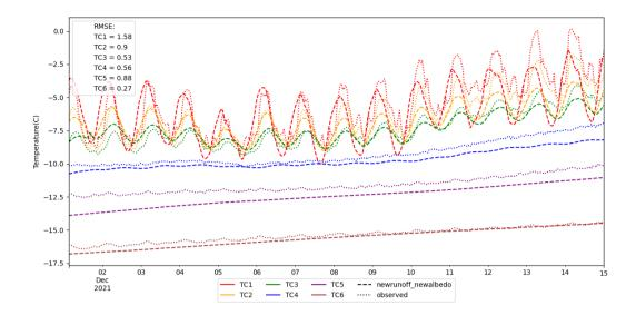
Figure 9. Modelled internal ice temperatures from newrunoff\_newalbedo for 1-15 December 2021. Thermocouples were initially deployed at six different depths: 0.05, 0.1, 0.2, 0.5, 1.0 and 2.0 meters. Note that the measurements are not at a constant depth with time as the sensors were melting out over the period. This shows diurnal variability at shallower depths and the seasonal warming wave below.
