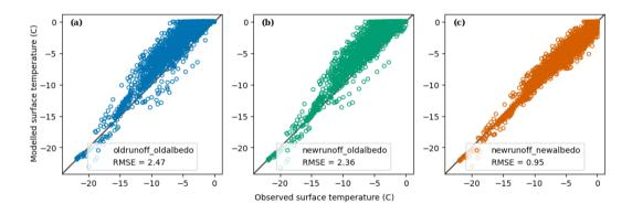
Figure 8. A scatter plot with modelled surface temperatures vs. observed surface temperatures for the three models from 1 December 2021 through to 28 February 2022.
