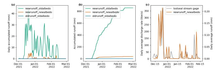
Figure 12. (a) Daily accumulated runoff and (b) cumulative runoff from the three model runs from 1 December 2021 - 28 February 2022. (c) Daily average discharge from the lost seal Lost Seal stream gauge (grey) compared to modelled daily average runoff (orange) from newrunoff newalbedo.
