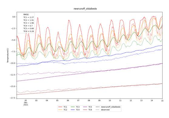
**Figure A2.** Modelled internal ice temperatures from newrunoff\_oldalbedo over the first two weeks of December. Thermocouples were initially deployed at six different depths: 0.05, 0.1, 0.2, 0.5, 1.0 and 2.0 meters. Note that the measurements are not at a constant depth with time as the sensors were melting out over the period.
