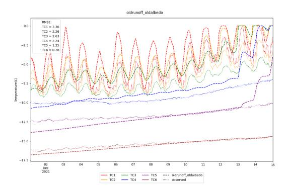
**Figure A1.** Modelled internal ice temperatures from oldrunoff\_oldalbedo over the first two weeks of December. Thermocouples were initially deployed at six different depths: 0.05, 0.1, 0.2, 0.5, 1.0 and 2.0 meters. Note that the measurements are not at a constant depth with time as the sensors were melting out over the period.
