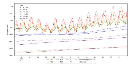
Figure 9. Modelled internal ice temperatures from newrunoff\_newalbedo over the first two weeks of for 1-15 December -2021. Thermocouples were initially deployed at six different depths: 0.05, 0.1, 0.2, 0.5, 1.0 and 2.0 meters. Note that the measurements are not at a constant depth with time as the sensors were melting out over the period. This shows diurnal variability at shallower depths and the seasonal warming wave below.
