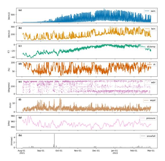
**Figure 3.** (a) Average hourly incoming shortwave radiation, incoming longwave radiation, surface temperature, relative humidity, wind direction, wind speed, <u>surface</u> pressure and snowfall measured at COHM AWS (1 August to 30 November 2021) and CWG AWS (1 December 2021 to 28 February 2022). Pressure is from the Antarctic Mesoscale WRF Prediction System (AMPS) for the first period as it was not measured at COHM AWS.
