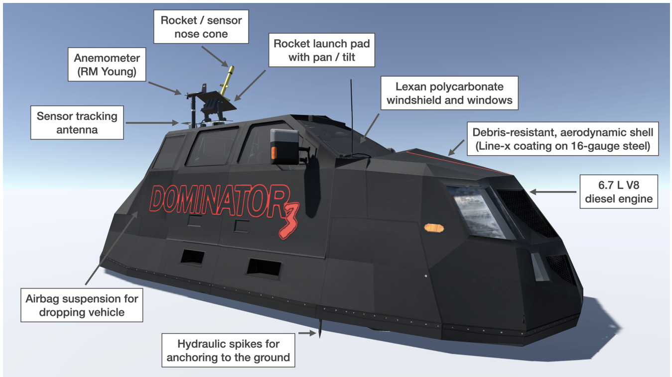
Figure 5. Dominator 3 storm chasing vehicle (credit: OUTBRK).
