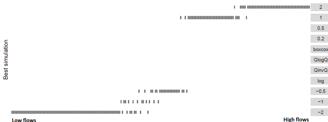
Figure 6. Identification of the simulation with the most number-1 ranks for the 325 catchments and for 200 intervals ordered by increasing observed streamflows. To provide this analysis, the output of Fig. 3f is used, and for each interval, the total of number-1 ranks is cumulated over the 325 catchments to identify the simulation with the most number-1 ranks. The GR4J model is used and is calibrated with NSE. Results are shown for the calibration period. The \lambda value for the Box–Cox transformation is 0.25.
