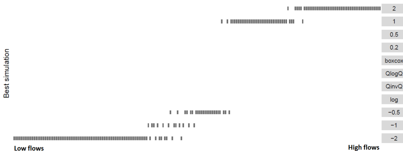
Figure 6. Identification of the simulation with the most rank 1 for the 325 catchments and for 200 intervals ordered by increasing observed streamflows. To provide this analysis, the output of Fig. 3f is used, and for each interval, the number of number 1 ranks is cumulated over the 325 catchments to identify the simulation with the most number 1 ranks. The GR4J model is used and is calibrated with NSE. Results are shown for the calibration period.
