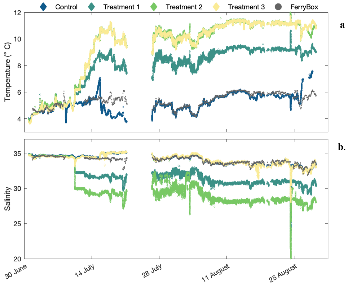
588 Figure 3. Mean (across triplicated mesocosms) temperature (°C; a ) and salinity ( b ) values 589 measured every minute over a 60 d period (including 6 day period before the start of the 590 experiment) for the control (blue), and for treatments 1 – 3 (dark green, light green, and yellow, 591 respectively).
