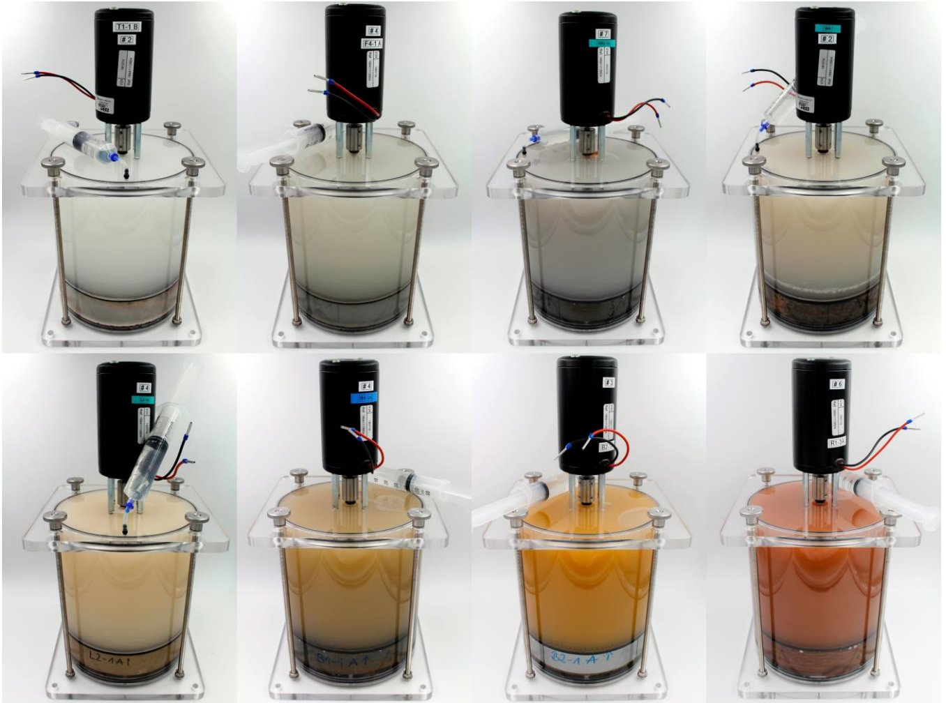
Figure 2: Erosion mills in use for experiments, with specimens from different lithologies. The turbidity indicates the concentration of erosion products in the water. Top row: Massenkalk (Unit 15) T1-1B, Lower Freshwater Molasse (Unit 2) F4-1A, Stafflegg Formation, Beggingen Member (Unit 4) GR2-1A, Murgtal-Gneisanatexit-Formation (Unit 18) W-4A. Bottom row: Schinznach Formation, Stamberg Member (Unit 8) L2-1A, Passwang Formation (Unit 1) B1-1A and B2-1A, Klettgau Formation, Ergolz Member (Unit 14) R1-3A.
