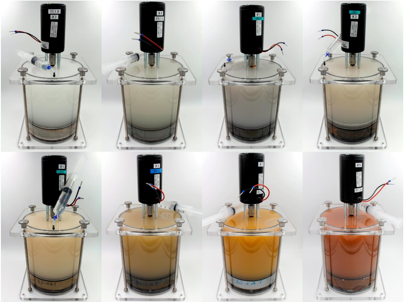
130 Figure 2: Erosion mills in use for experiments, with specimens from different lithologies. The turbidity indicates the concentration of erosion products in the water. Top row: Massenkalk (Unit 15) T1-1B, Lower Freshwater Molasse (Unit 2) F4-1A, Stafflegg Formation, Beggingen Member (Unit 4) GR2-1A, Murgtal-Gneisanatexit-Formation (Unit 18) W-4A. Bottom row: Schinznach Formation, Starnberg Member (Unit 8) L2-1A, Passwang Formation (Unit 1) B1-1A and B2-1A, Klettgau Formation, Ergolz Member (Unit 14) R1-3A.
