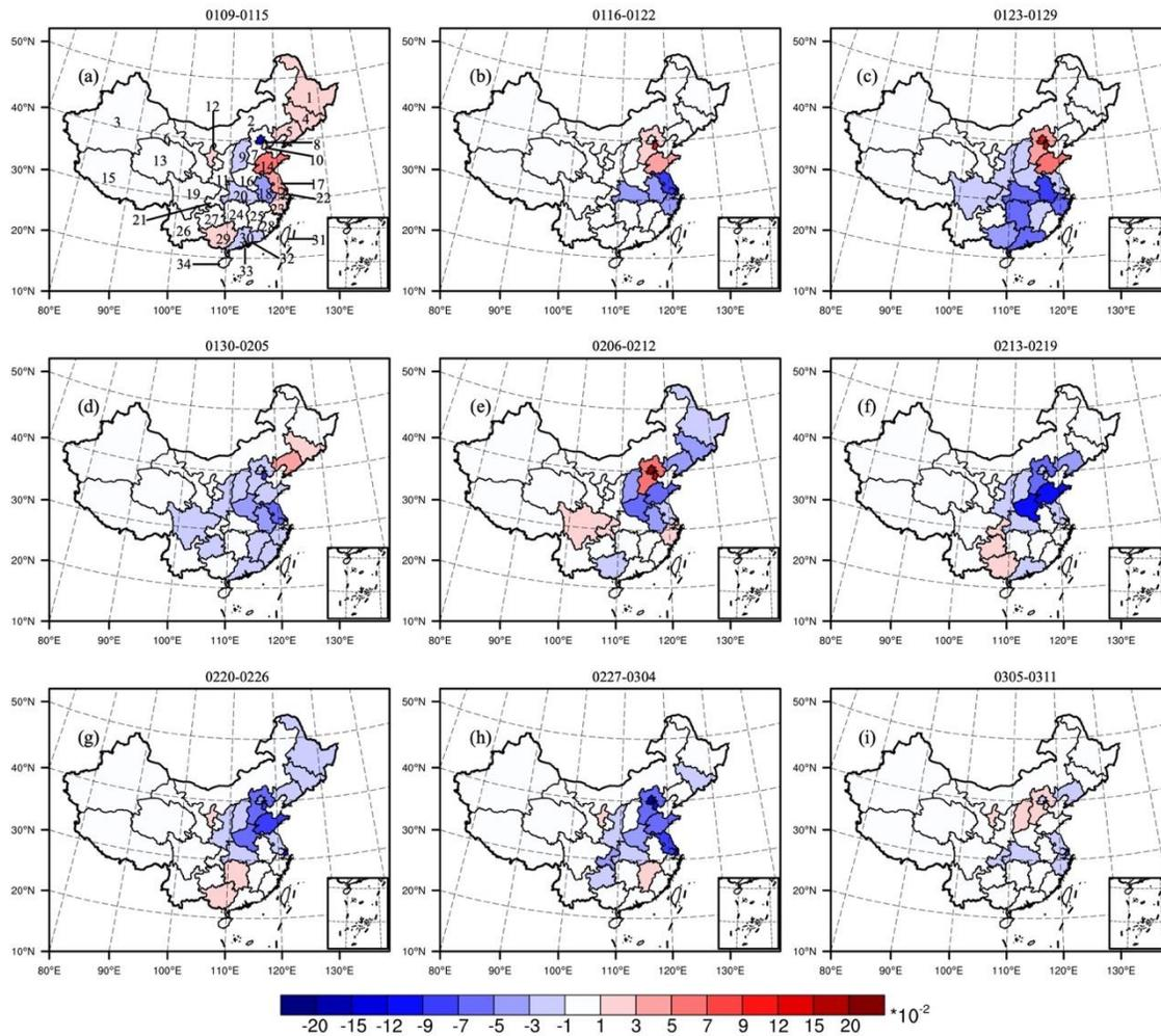
750 **Figure 12.** Mean spatial distributions of PM<sub>2.5</sub> emission differences ( $\mu\text{g}\cdot\text{m}^{-2}\cdot\text{s}^{-1}$ ) between year
