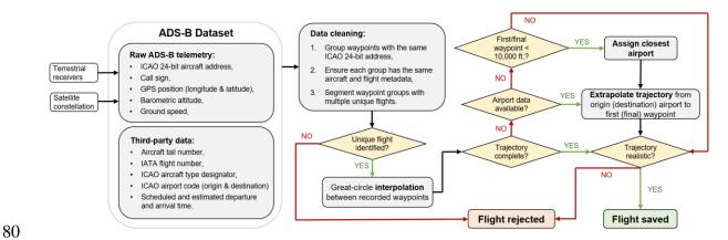
Figure S2: Data cleaning and trajectory completion workflow that is used to process the raw ADS-B
