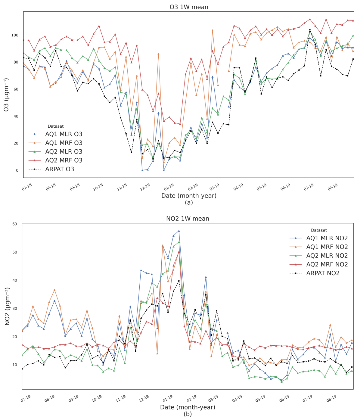
Figure S10. Trend analysis of 7-day average O 3 and NO 2 concentrations measured at the validation site by the calibrated AQ1 and AQ2 stations compared to the ARPAT reference station (17 June 2019–22 August 2019).
