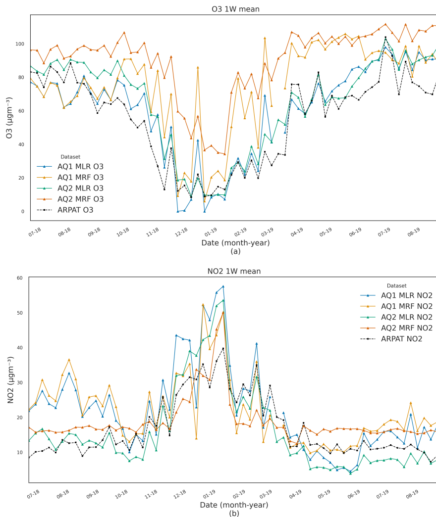
Figure 8. Trend analysis of 7-day average O 3 and NO 2 concentrations measured at the validation site by the calibrated AQ1 and AQ2 stations compared to the ARPAT reference station (17 June 2019–22 August 2019)
