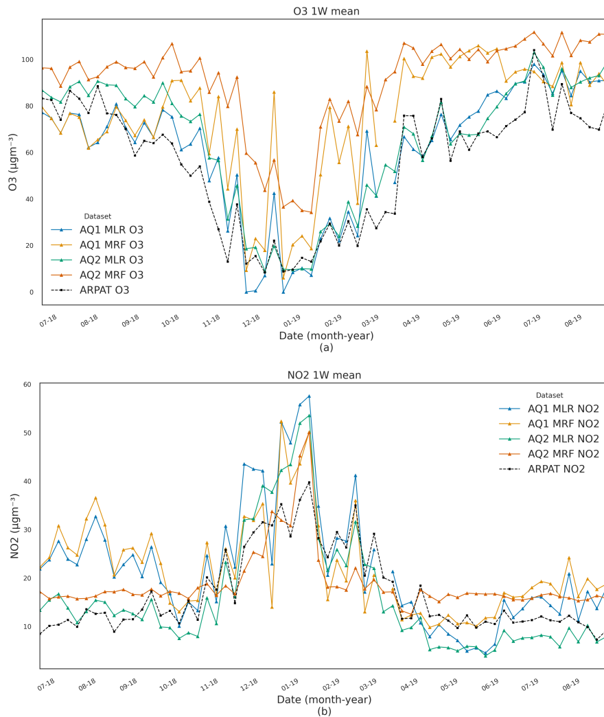
Figure 8. Taylor diagrams Trend analysis of the pre7-deployment MLR and MRF calibrated models assessed against the ARPAT reference station for O 3 (a) day average O 3 and NO 2 (b) NO 2 concentrations. The Taylor diagram (Rochford, 2016) consists of a polar plot in which the radial distance from the origin represents the standard deviation of predictions, and measured at the angle represents validation site by the correlation between predictions calibrated AQ1 and observations. Models that agree well with observations lie closer AQ2 stations compared to the red line. CRMSD is a relative measure of model fit, providing a normalized measure of the deviation from the actual values. This deviation is normalized by the standard deviation of the ARPAT reference values, which allows a fair comparison of models' performance. station (17 June 2019–22 August 2019)
