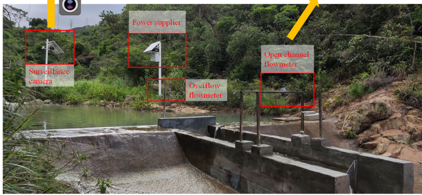
132 Figure 1. Camera setup. The camera is set on the left bank of the stream, about 3 m
