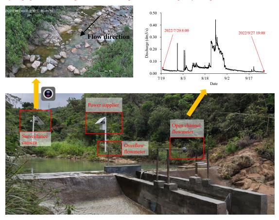
Figure 1. Camera setup. The camera is set on the left bank of the stream, about 3 m above the water surface, and 8 m upstream of a gauging weir. The top right panel demonstrates the changes in the flowmeter's discharge during the measurement period.
