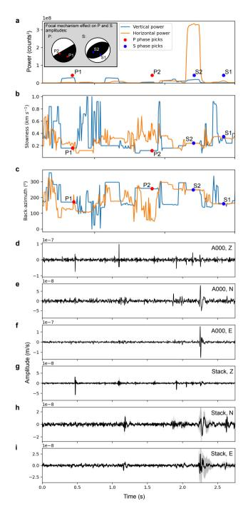
**Figure 3.** Example of array phase detection and association performance. a. Plot of power-beam-power and peaks associated with phase arrivals for two events. n of an event alysis (FTAN) Inset diagram shows possible focal mechanism effects mechanisms that could cause the observed P- and S- amplitudes. b-dd-f. Waveforms arriving at centre array station. e-gg-i. Mean of stacked and time-shifted waveforms for the entire array, using the slowness and back-azimuth of event 2 in (ab) (c).
