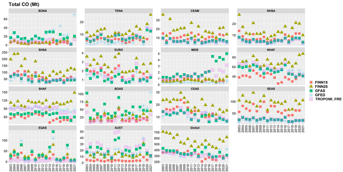
Figure 10. To illustrate the trend of CO fire emissions the sum of all 5 inventories (FINN1.5, FINN2.5, GFED v4.1, GFAS and “TROPOMI-GFAS”) is shown for the different geographical regions between 2003 and 2021.
