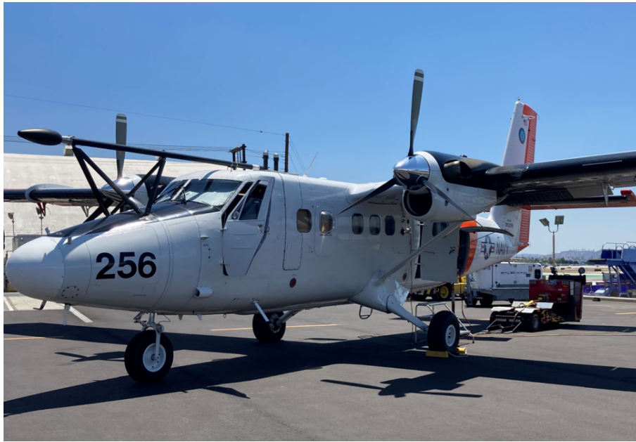
Figure S1. NPS Twin Otter aircraft, including the mounted inlet for air sampling.
