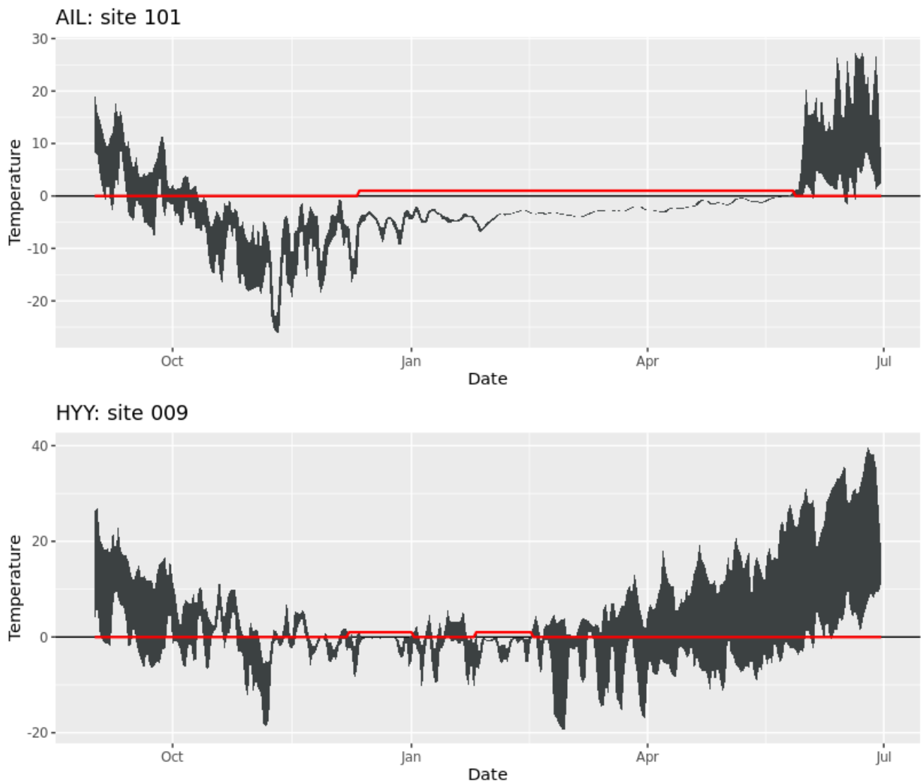
Figure A1. Examples of detecting snow cover duration from the temperature time series. The dark grey color shows daily maximum and minimum values of near-surface air temperatures (+15 cm) and the red line indicates when the algorithm detects snow cover (0 = no snow cover, 1 = snow cover).
