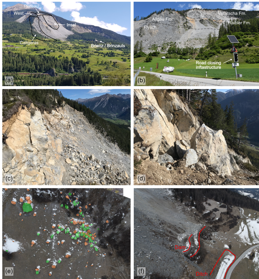
Figure 2. Photos from the study site. (a) View from Ruteira (above Tiefencastel see Fig. 1c) on the complete mountain slope deformation with marked compartments of Brienz/Brinzauls, looking NNE. (b) View on the rockfall release, transport and deposition areas from the Doppler radar location and main road, looking north with indicated geological contacts. The shadow area with meadow and main road is in the foreground, trees on the rockfall dam are located between the shadow area and talus cones. (c) and (d) Upper sector of release area showing fractured Arlberg dolomite, looking east from the NW corner of the Insel compartment. (e) Deposited blocks in the shadow area. Green blocks were deposited before 21 April 2022. Orange colored blocks were deposited in the period between 21 April and 30 January 2023. (f) Side view of the partially filled rockfall dam and the adjacent shadow area.
