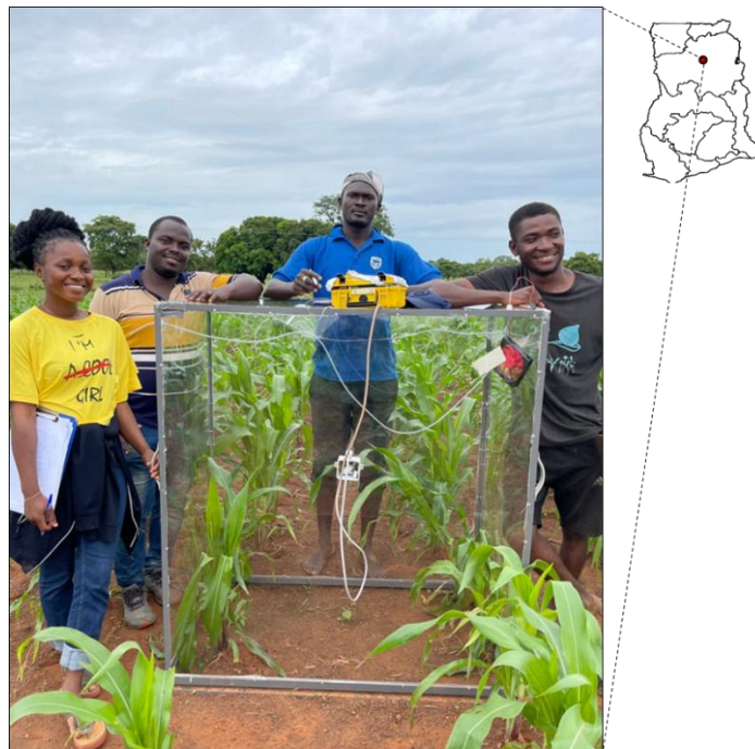
Figure 4: Transparent (NEE) manual closed chamber measurement at CSIR-SARI experimental field, used for field trial application of the developed, low-cost CO 2 and ET flux measurement device, near the city of Nyankpala, Northern Ghana (9°24'15.9" N, 01°00'12.1" W).
