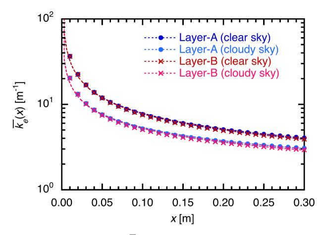
Figure 3: Broadband flux extinction coefficient  $\overline{k_e}(x)$  of bare ice as a function of ice thickness x for clear and cloudy sky conditions and employed data sets of  $k_e(\lambda)$  for Layers A and B reported by Cooper et al. (2021). Calculated values are indicated by symbols and dashed curves represent approximation equations fitted by power regression equations.
