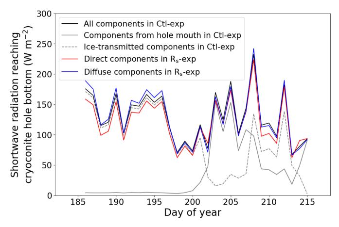
Figure 10: Daily mean temporal changes in direct and diffuse components of shortwave radiation reaching the cryoconite hole (CH)
