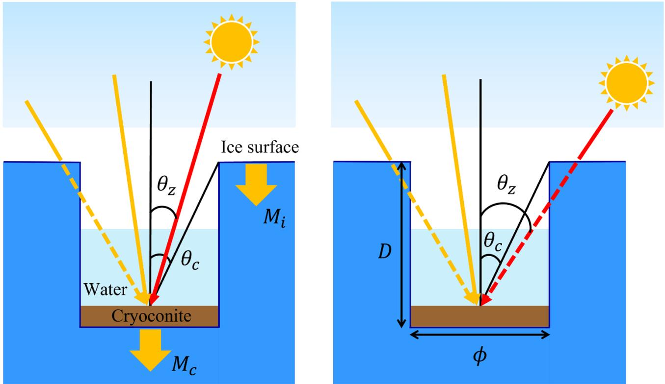
695 **Figure 1: Concept of the cryoconite hole model (CryHo).** Heat balances at the surface and cryoconite hole bottom are independently
