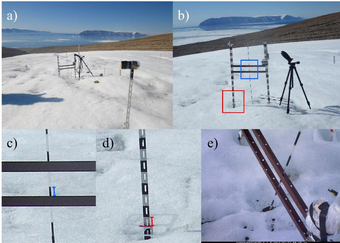
740 Figure 6: (a) Device for monitoring the cryoconite hole (CH) depth at Site 2, (b) sample image to quantify the CH depth, which was
