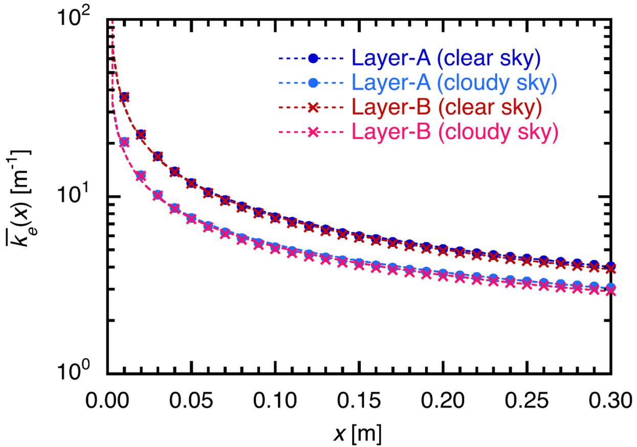
Figure 3: Broadband flux extinction coefficient  $\bar{k}_e(x)$  of bare ice as a function of ice thickness  $x$  for clear and cloudy sky conditions and employed data sets of  $k_e(\lambda)$  for Layers A and B reported by Cooper et al. (2021). Calculated values are indicated by symbols and dashed curves represent approximation equations fitted by power regression equations.
