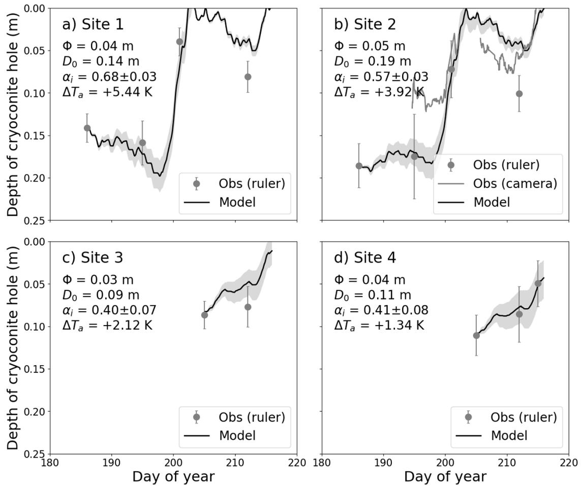
**Figure 7: Temporal changes in cryoconite hole (CH) depth at (a) Site 1, (b) Site 2, (c) Site 3, and (d) Site 4 in 2014. The CH constants, ice surface albedo and air temperature correction are described in each panel. The black solid line and shading indicate model results using average values and standard deviations of ice surface reflectance, which is assumed to be  $\alpha_i$ , as shown in Table 2. The missing grey solid line in panel b denotes the CH collapse period.**
