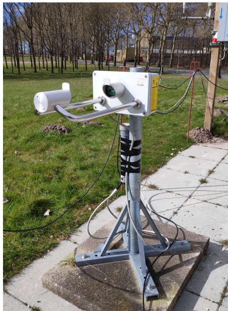
Figure 4: Thies Laser Precipitation Monitor(LPM) at DTU Risø campus.
