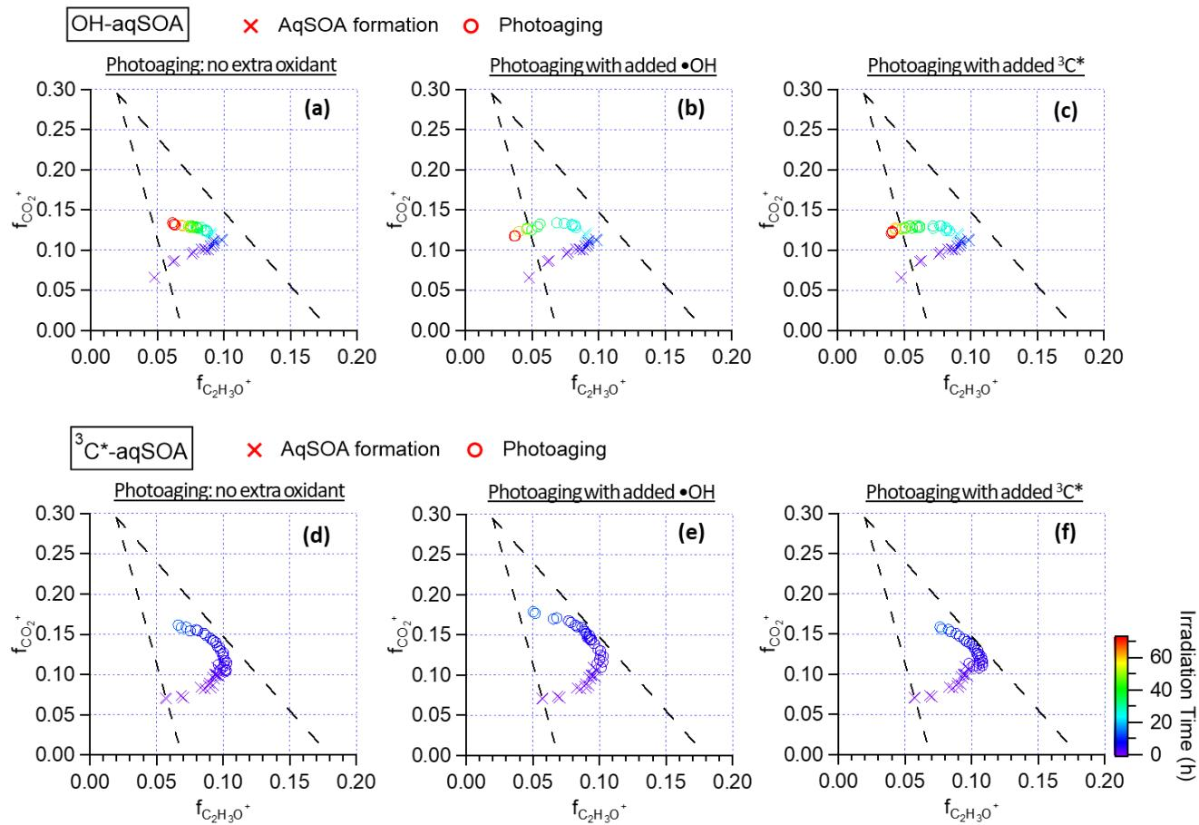
**Figure S8.** Triangle plots ( $f_{CO_2^+}$  vs  $f_{C_2H_3O^+}$ ) that depict the evolution trends of the  $\bullet OH$ -aqSOA and  $^3C^*$ -aqSOA under different photoaging conditions.
