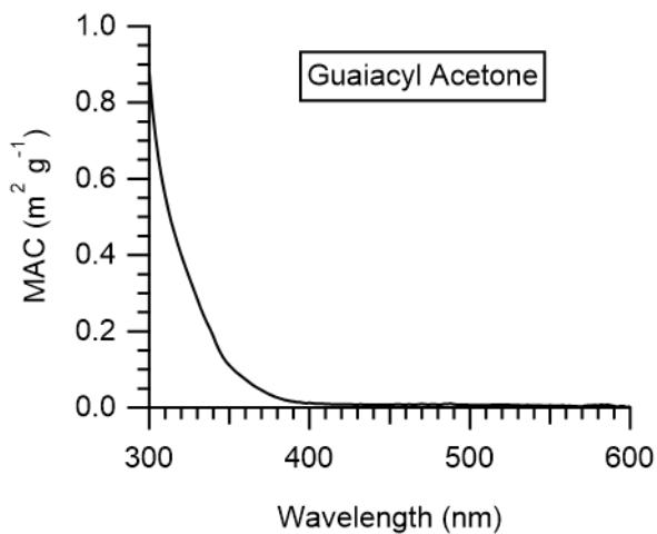
**Figure S5.** Mass absorption coefficient spectra of guaiacyl acetone.
