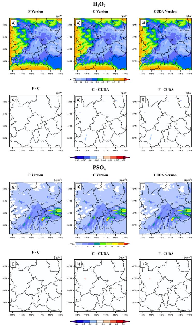
718 **Figure 7.** H<sub>2</sub>O<sub>2</sub> and PSO<sub>4</sub> concentrations output by the CAMx model for the Fortran, standard C,
