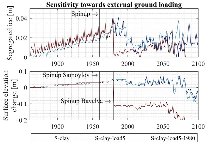
Column-accumulated segregated ice and surface elevation changes on the reference date August 31 for the model scenarios *S-clay*, *S-clay-load5* and *S-clay-load5-1980*. A load that is acting on the soil column from the beginning of the simulation (*S-clay-load5*) suppresses ice segregation. A load that is added during thaw consolidation (*S-clay-load5-1980*) accelerates the process and the ground surface subsides faster.
