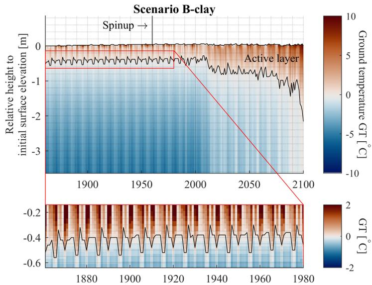
Ground temperatures on the reference date August 31 for the model scenario B-clay. *The detailed plot shows the ground temperatures at the permafrost table during the spin-up, where ice segregation takes place.*
