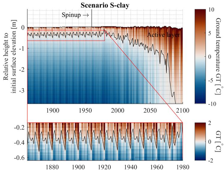
Ground temperatures on the reference date August 31 for the model scenario S-clay. *The detailed plot shows the ground temperatures at the permafrost table during the spin-up, where ice segregation takes place.*
