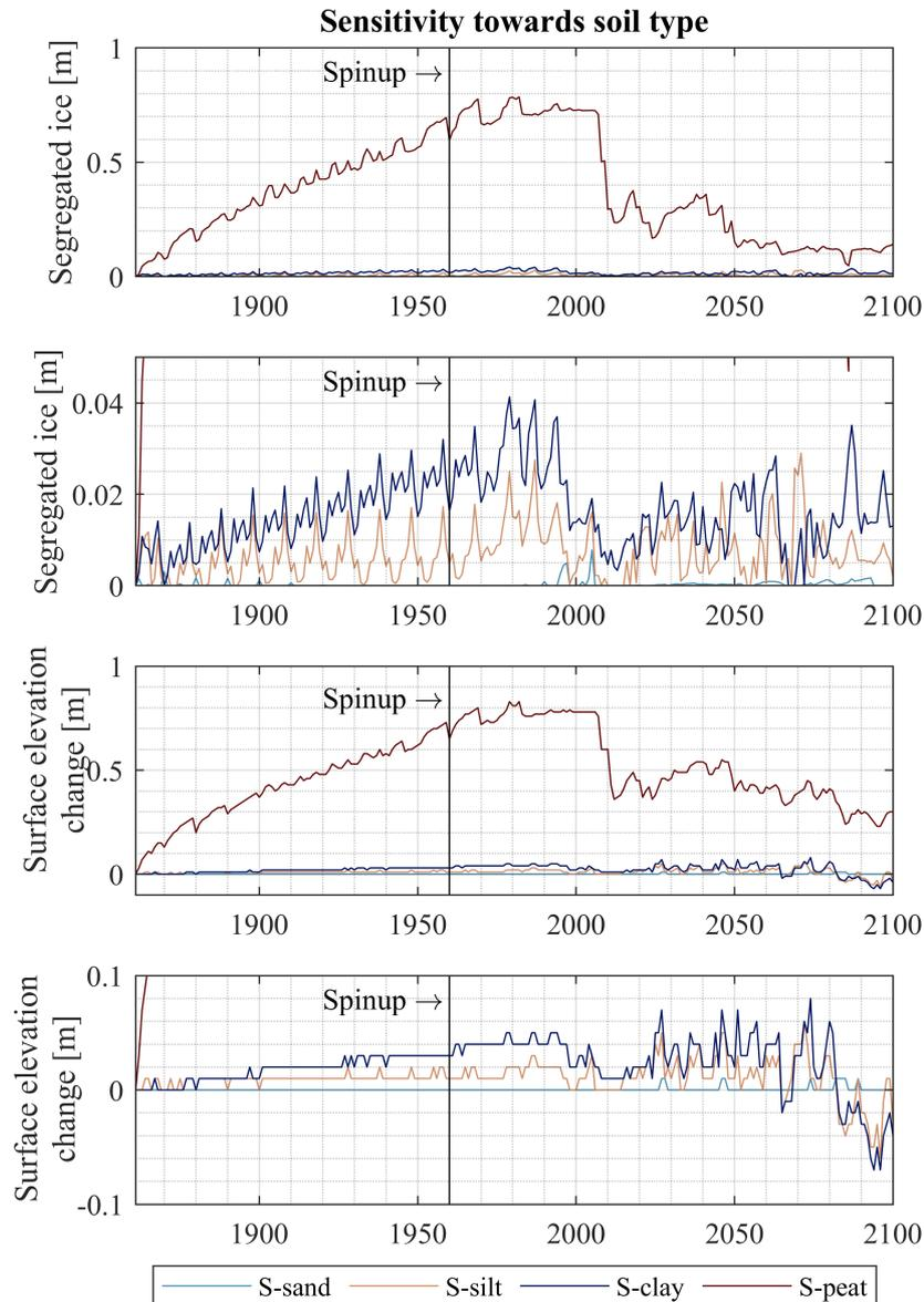
220 *Column-accumulated segregated ice and surface elevation changes on the reference date August 31 for the model scenarios S-sand, S-silt, S-clay and S-peat. With decreasing particle diameter, the soil builds up more segregated ice under equal conditions. Peat soils form substantially more ground ice than mineral soils.*
