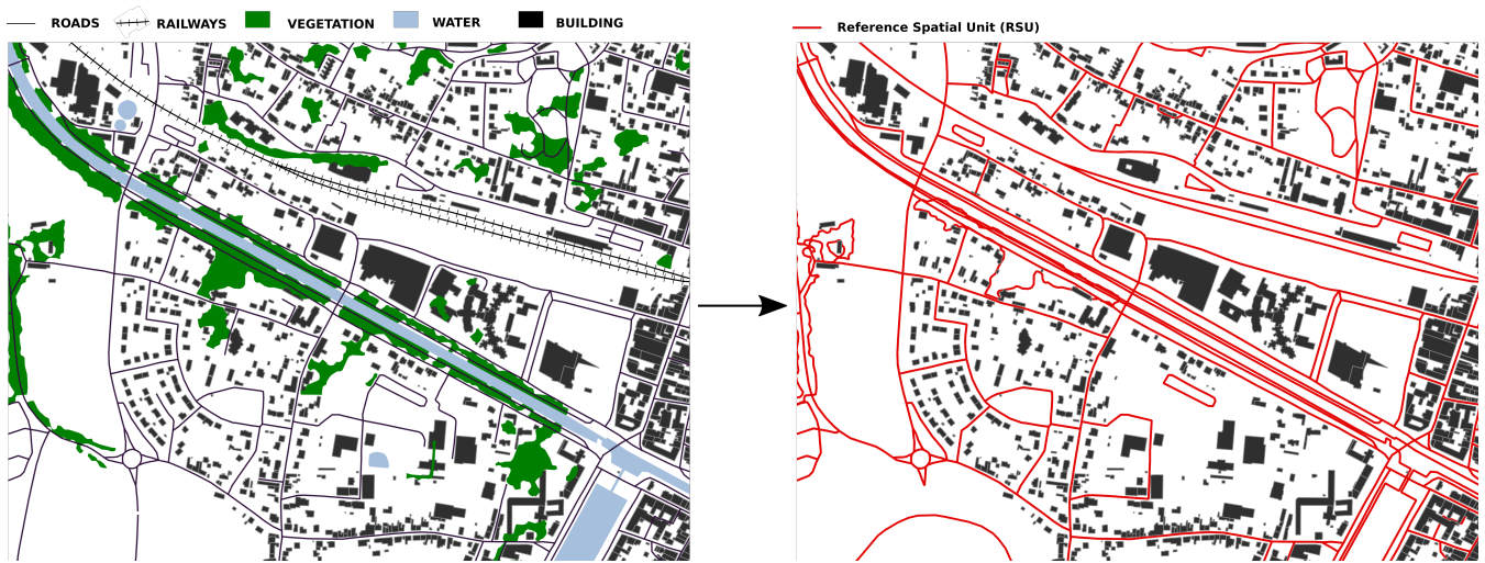
Figure 1. Illustration of the method to produce the Reference Spatial Units using BDT data
