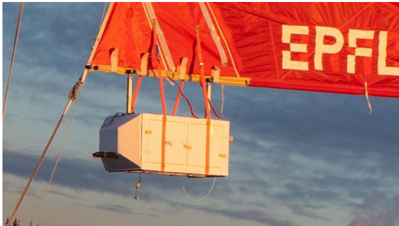
Figure 1: Picture of the MoMuCAMS payload attached to the helikite. Two aluminum bars connected directly to the helikite's structure ensure stability of the payload. Two additional cargo straps provide additional safety for the payload attachment. The system remains very stable, even at winds above 15 \text{ m s}^{-1} .
