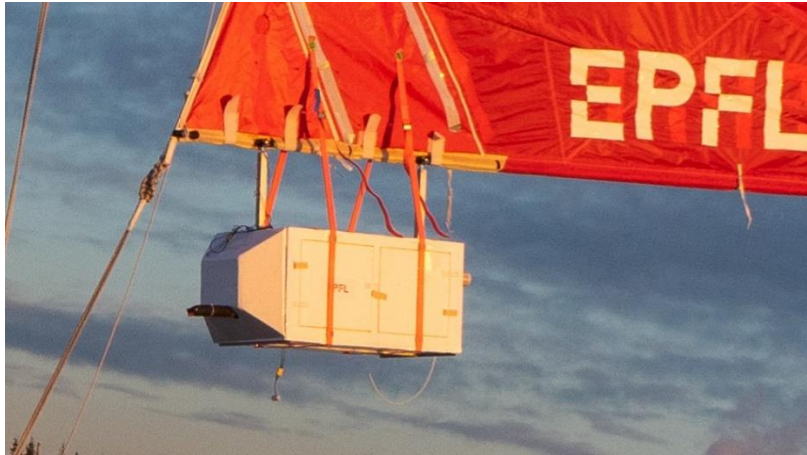
1115 Figure 1: Picture of the MoMuCAMS payload attached to the helikite. Two aluminum bars connected directly to the helikite's structure ensure stability of the payload. Two additional cargo straps provide additional safety for the payload attachment. The system remains very stable, even at winds above 15 m s -1 .
