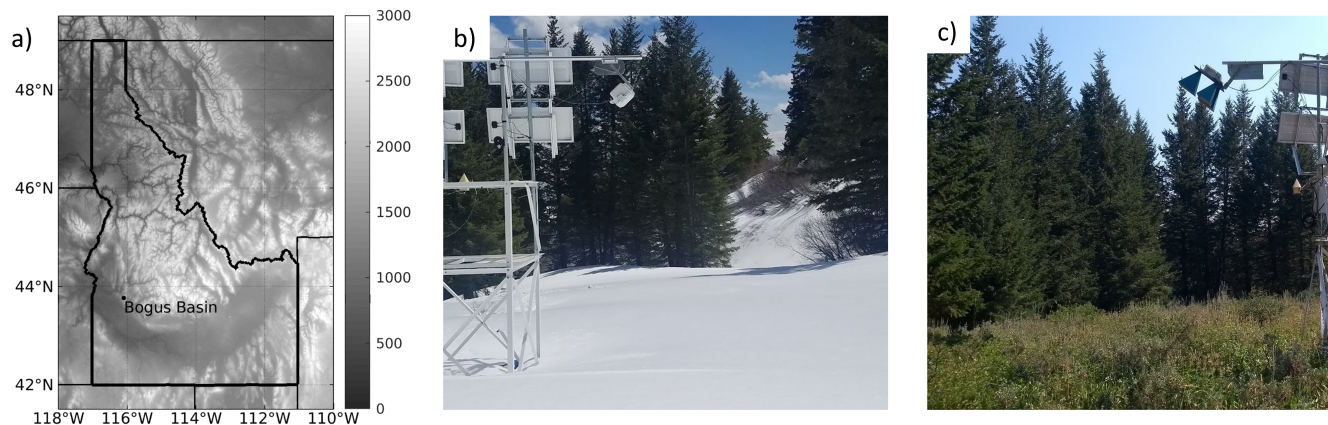
Figure 1. Study site. (a) The location of the site in Idaho (US), with the background representing the elevation (m) from the Shuttle Radar Topography Mission (Farr et al., 2007). (b) The site in winter with the box containing the radar with tapered slot antennas as used in winter 2021-2022. (c) The site and its vegetation in summer during installation of the radar with horn antennas used in winter 2022-2023.
