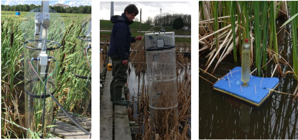
Figure 3 Automated chamber (left), manual chamber (middle), and bubble trap (right), used for measuring fluxes.
