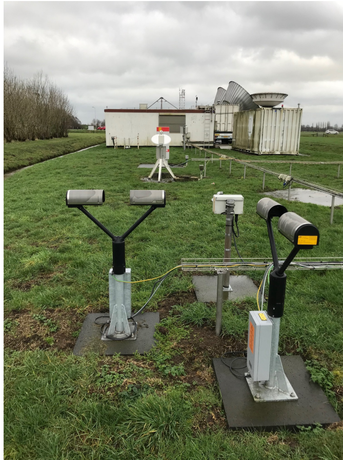
Figure 1. Parsivel 2 disdrometers at the Cabauw site for atmospheric research in the Netherlands. The micro-rain radar is visible in the background.
