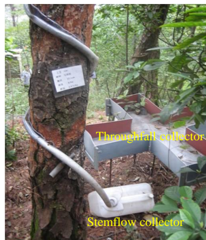
Fig. S1 Collecting equipment and their locations of throughfall and stemflow
