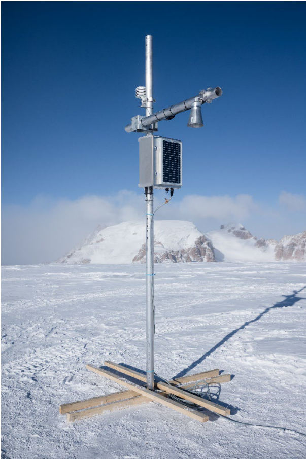
Fig 1: Grigoriev firn station on 8 February 2018, immediately after installation. Distance from snow surface to the horizontal boom is 2.74 m.
