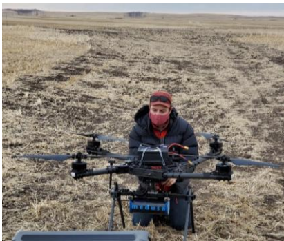
Figure 1: Medusa MS-1000 mounted on a FreeFly AltaX prior to survey November 6, 2020. Photo credit Anders Hunter.
