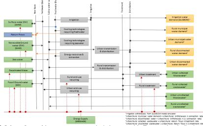
Figure 3: Reference System of the water system representation in the nexus module. The arrows show the direction of input/output of different technologies within the framework. Energy footprint of water system is tracked at different supply steps and infrastructure technologies.
