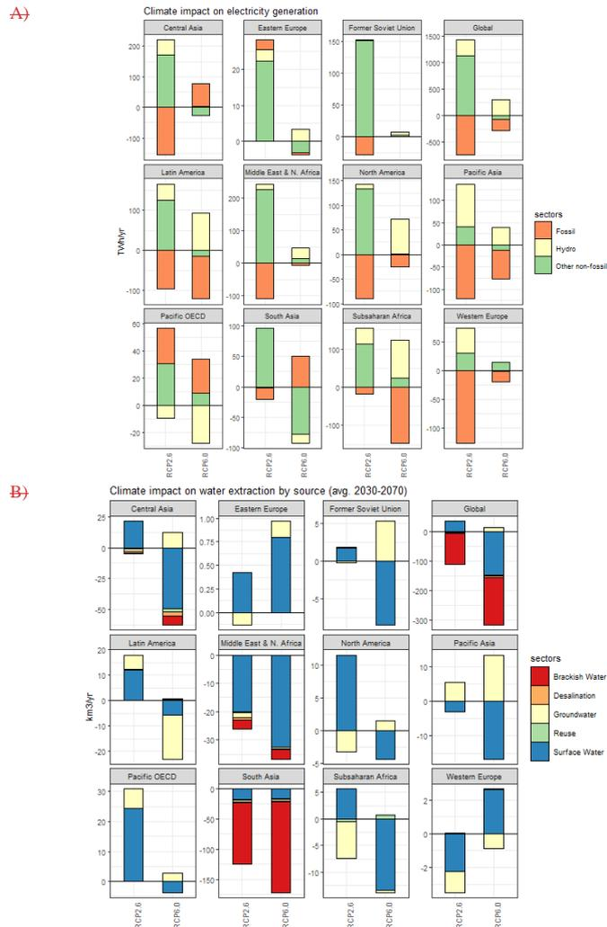
Figure 6 A) Climate impacts on electricity generation (TWh/yr.). The average of 2030-2070
