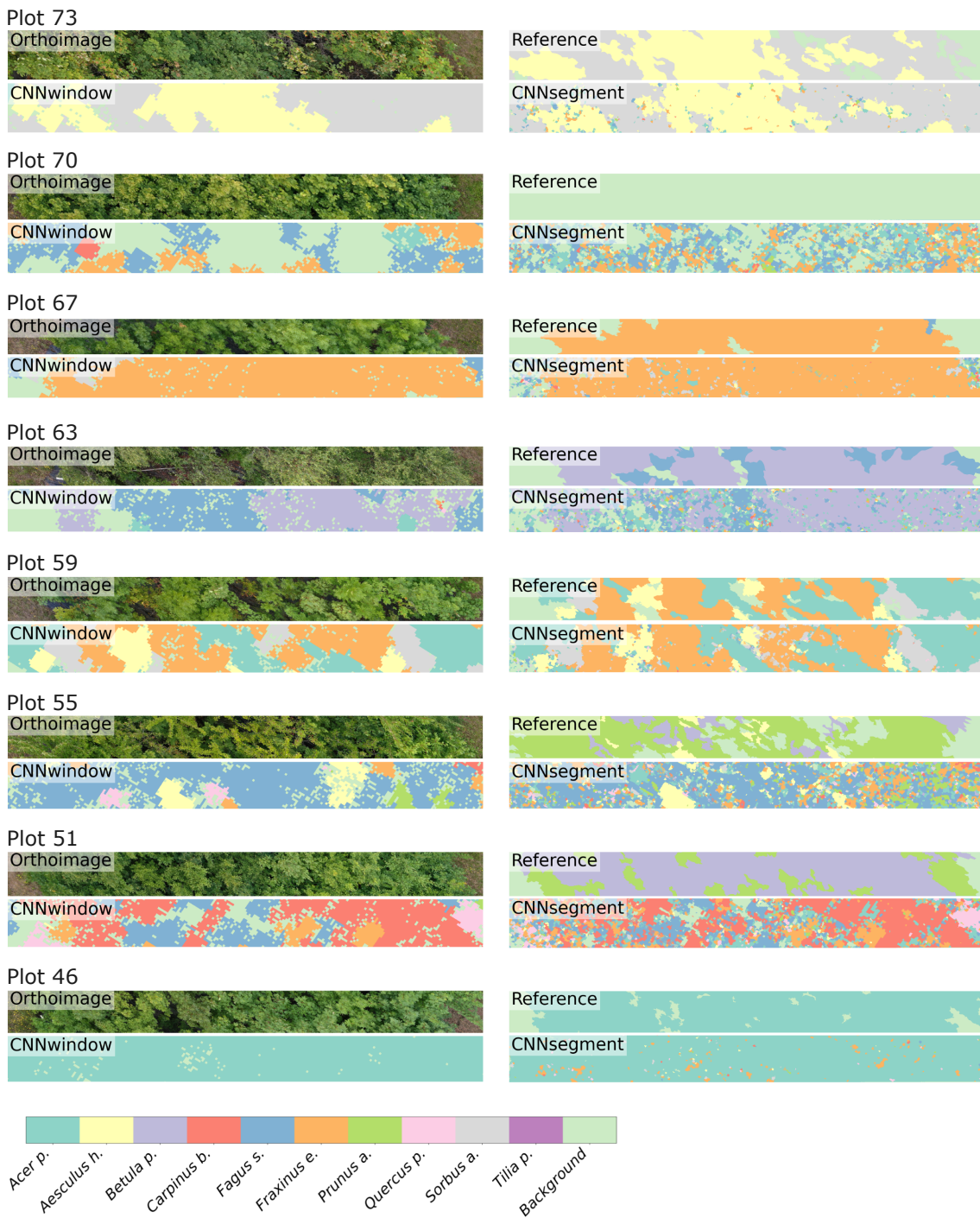
Figure A9: Transects of 2 m by 20 m of selected plots, including the orthoimage, the reference, CNN window predictions, and CNN segment predictions.
