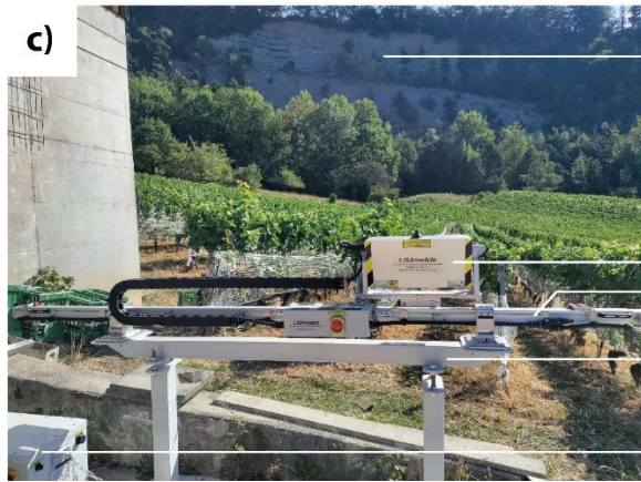
Figure 13 : Second real studied site: La Cornalle cliff. a) Location. b) Radar and target location on Google Earth image. c) Lisalab GB-InSAR installation.
