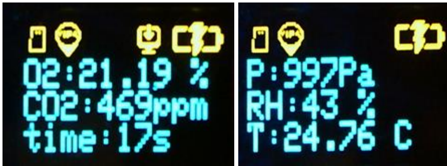
80 Figure 2. small 0.96", yet very readable, OLED display permuting screens with different useful information.
